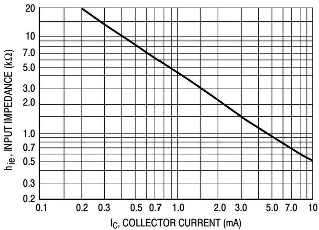
Figure 12. Input Impedance
