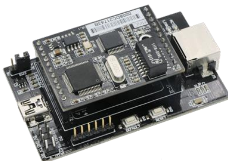
Figure 2-3 WIZS2E evaluation board
