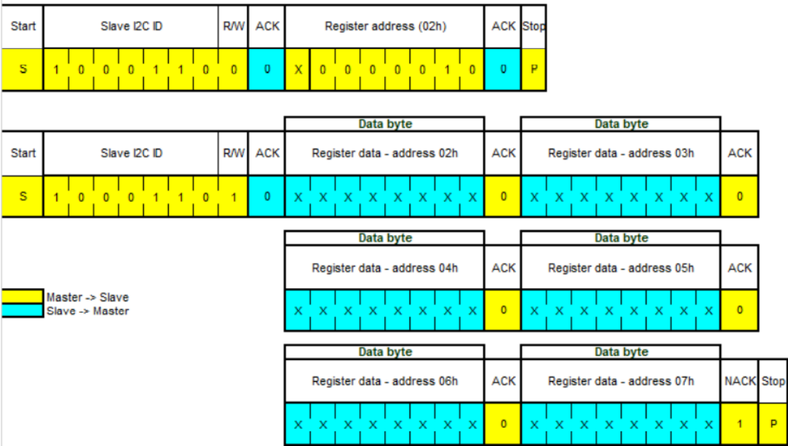
Figure 16: multi-byte read protocol with stop-start
