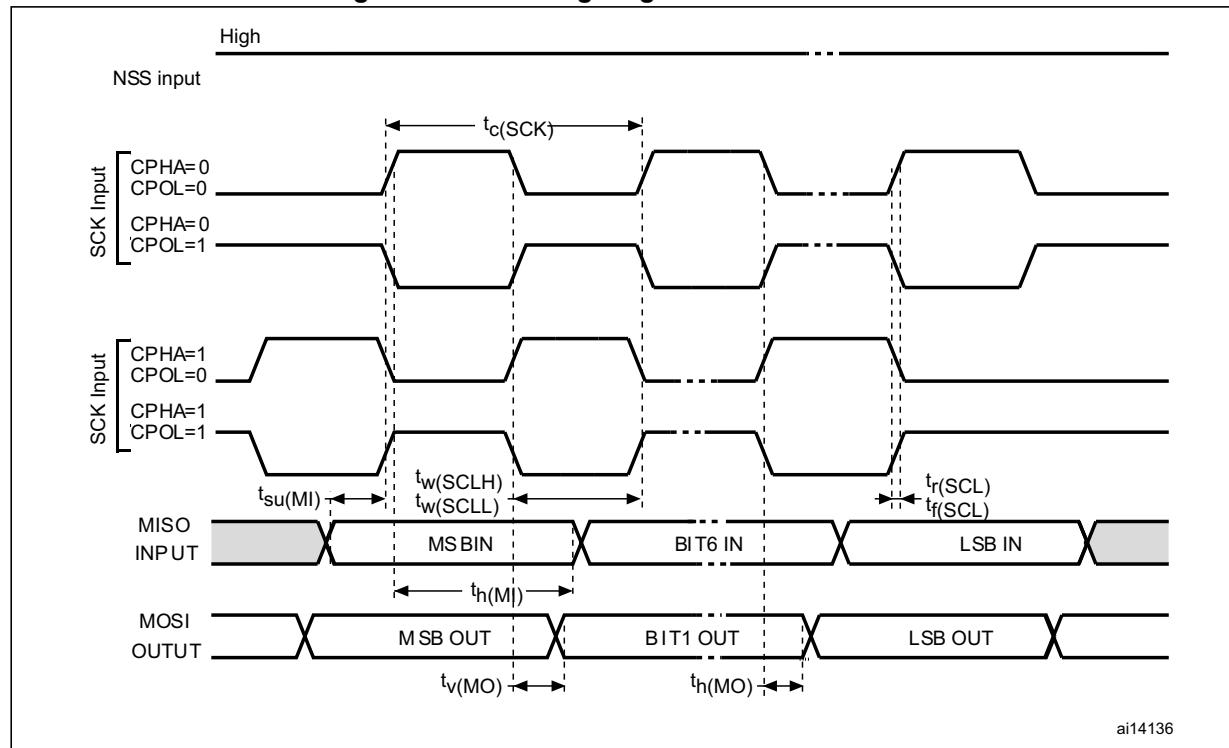
1. Measurement points are done at CMOS levels:  $0.3V_{DD}$  and  $0.7V_{DD}$ .
