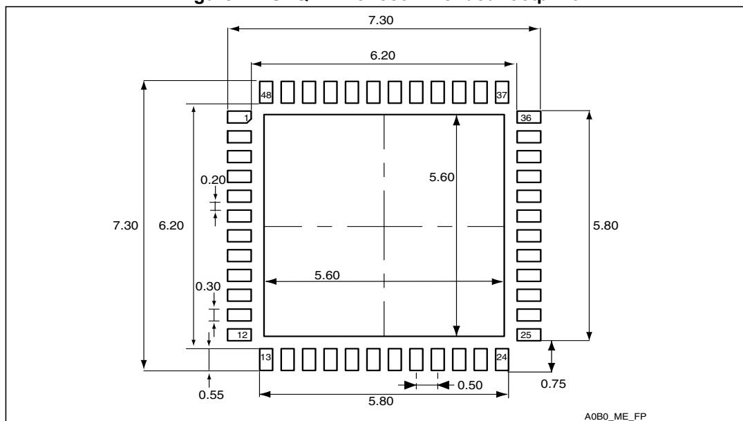
1. Dimensions are in millimeters.
