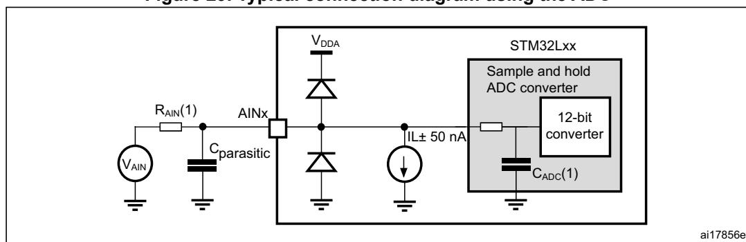
1. Refer to [Table 58: Maximum source impedance  \$R\_{\text{AIN max}}\$](#)  for the value of  $R_{\text{AIN}}$  and [Table 56: ADC characteristics](#) for the value of  $C_{\text{ADC}}$ .
