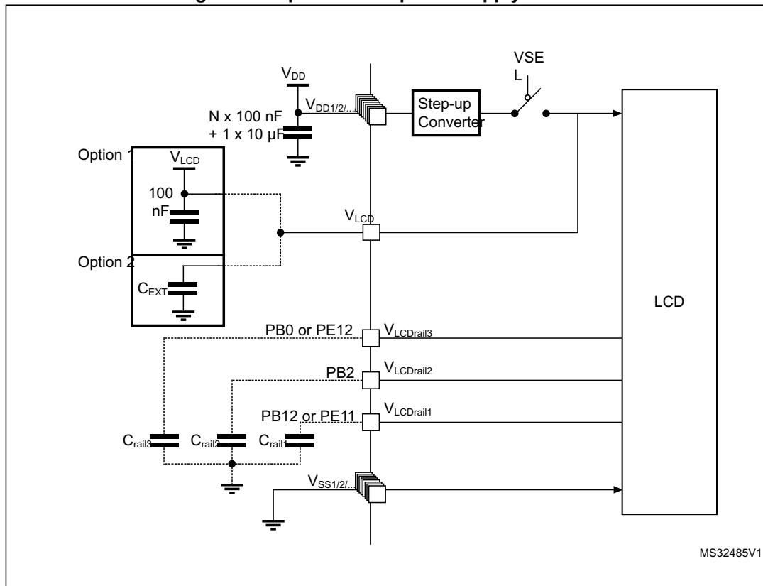
1. Option 1: LCD power supply is provided by a dedicated VLCD supply source, VSEL switch is open.
