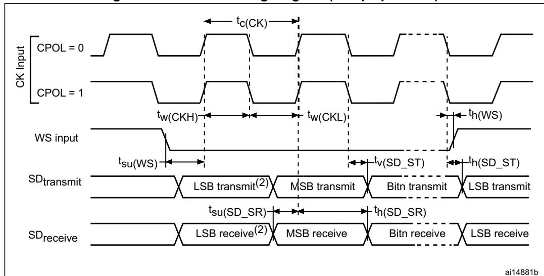
1. Measurement points are done at CMOS levels:  $0.3 \times V_{DD}$  and  $0.7 \times V_{DD}$ .
