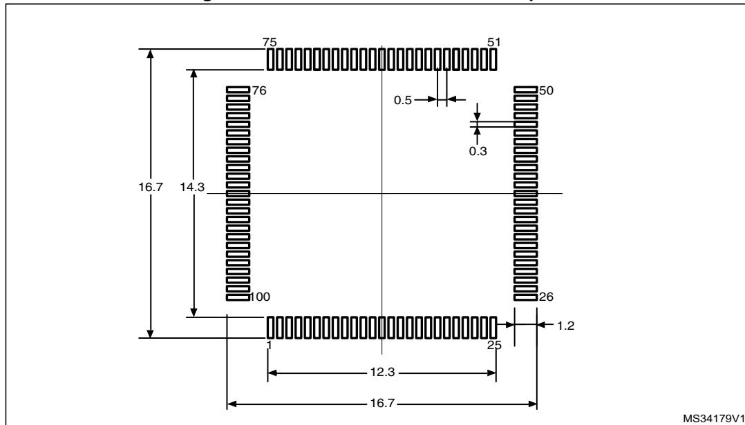
1. Dimensions are in millimeters.
