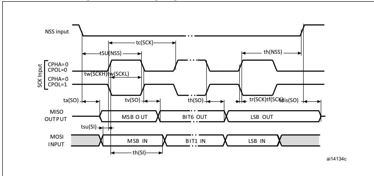
Figure 23. SPI timing diagram - slave mode and CPHA = 1<sup>(1)</sup>
