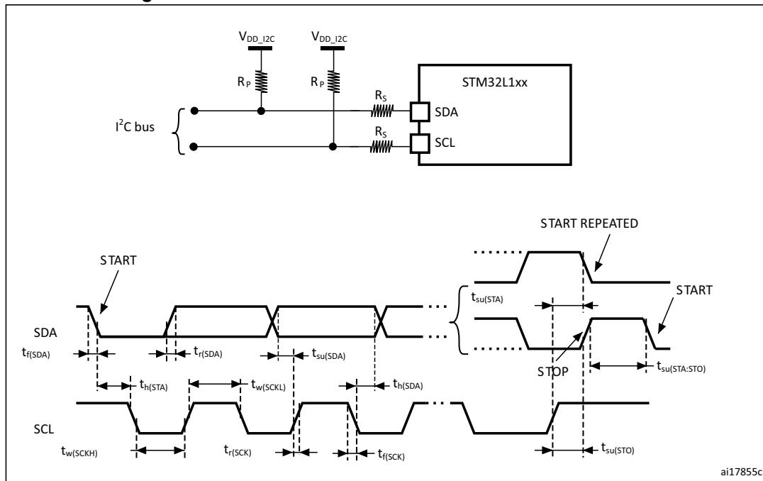
1.  $R_S$  = series protection resistor.
