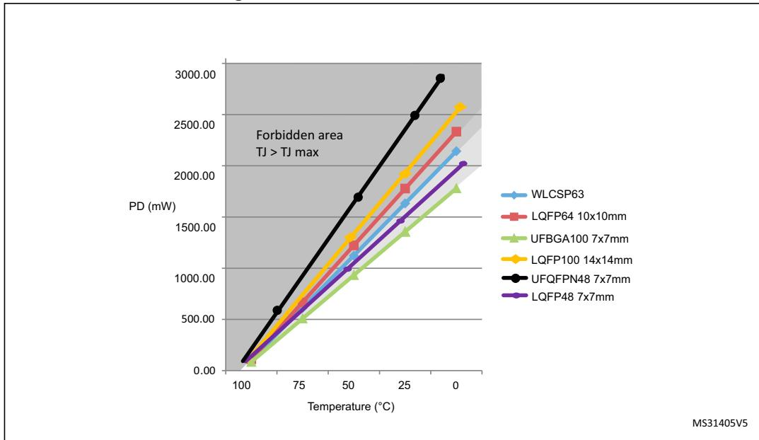
**Figure 48. Thermal resistance suffix 7**
