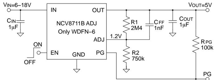
Figure 4. Adjustable Output Voltage Application with PG
