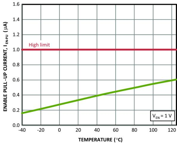
Figure 10. Enable Internal Pull-Up Current vs. Temperature
