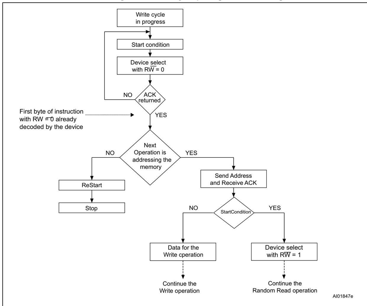
1. The seven most significant bits of the Device Select code of a Random Read (bottom right box in the figure) must be identical to the seven most significant bits of the Device Select code of the Write (polling instruction in the figure).
