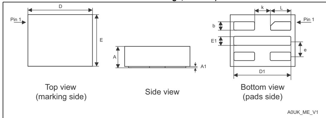
1. On the bottom side, pin 1 is identified by the specific pad shape and, on the top side, pin 1 is defined from the orientation of the marking: when reading the marking, pin 1 is below the upper left package corner.
