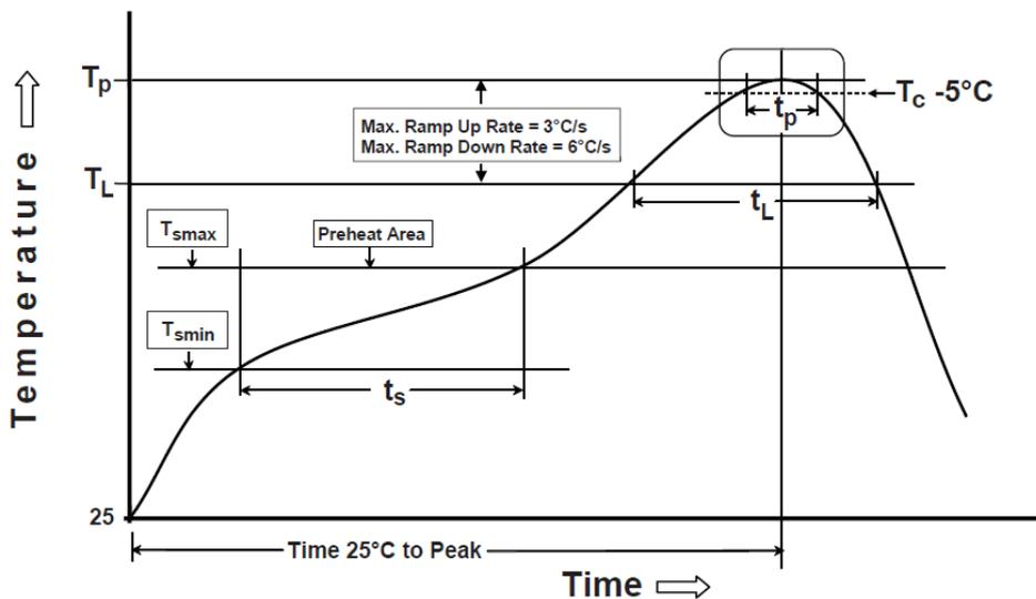
Soldering condition: Apply preheating at 120°C for 2-3 minutes. Finish soldering for each terminal within 3 seconds. If soldering iron temperature over  $270^\circ\text{C} \pm 10^\circ\text{C}$  for 3 seconds, it may cause component surface peeling or damage.
