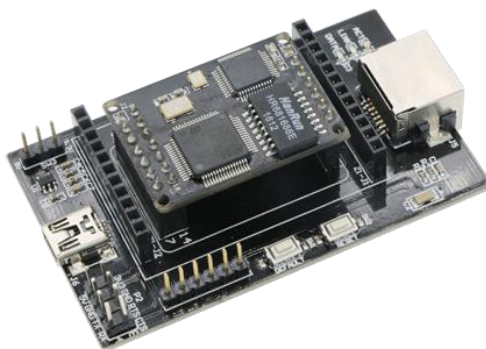
Figure 2-3 WIZS2E evaluation board
