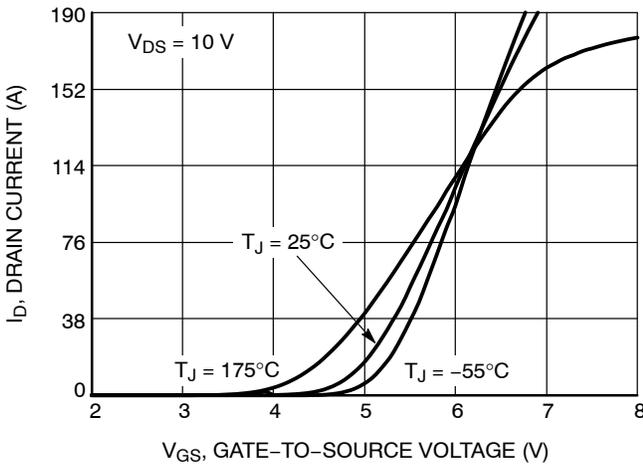
Figure 5. Transfer Characteristics
