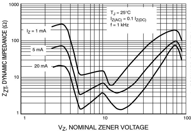
**Figure 5. Effect of Zener Voltage on Zener Impedance**
