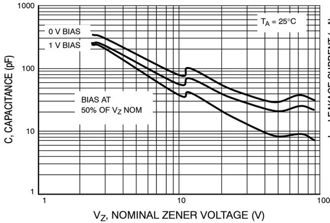
Figure 7. Typical Capacitance
