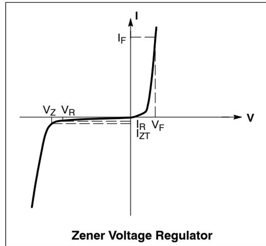
**ELECTRICAL CHARACTERISTICS** ( $T_A = 25^\circ\text{C}$  unless otherwise noted,  $V_F = 0.9\text{ V Max. @ } I_F = 10\text{ mA}$ )
