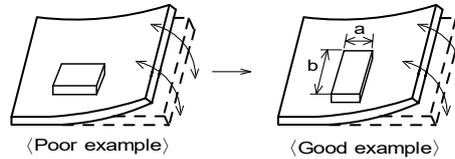
(2) Components location on PCB separation
