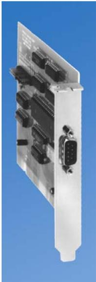
These computer brackets have been designed to accommodate a large variety of board sizes and heights. Available with tabs located properly for ESA/EISA or PCI formats. Blanks can be machined or stamped for prototype or low volume production. All brackets are nickel plated for a clean look and a protective finish. Standard cut-outs can be added to these blanks to suit your specific production needs. See page 118-119 for standard cut-outs and design worksheet.
