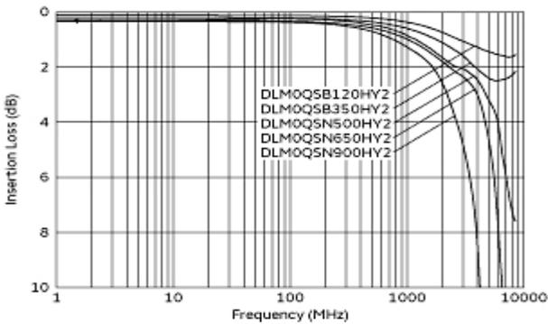
Differential Mode Transmission Characteristics (Typical Value)
