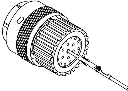
**IMPORTANT NOTE:** The stitching tool is not designed to pull the contact through; it is intended to ease the insertion process with high density connectors.
