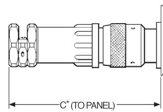
**Sealed Cable Clamps for Use With Neptune Circular Connectors**
