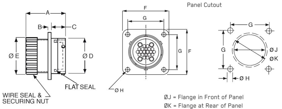
With Wire Seal and Securing Nut
