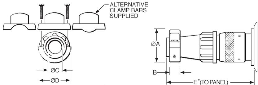
\* For disassembly, add 9,00 (.354) for Shell Sizes 10-16 & add 10,60 (.417) for Shell Sizes 18-24.
