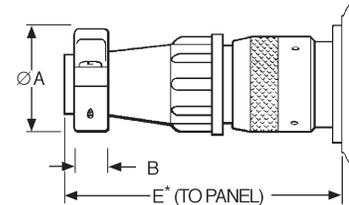
\* For disassembly, add 9,00 (.354) for shell sizes 14 and 16 and add 10,60 (.417) for shell size 24.
