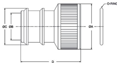
Heat Shrink Adapter for use with TNM Circular Connectors
