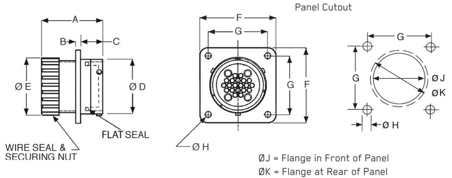
With Wire Seal and Securing Nut
