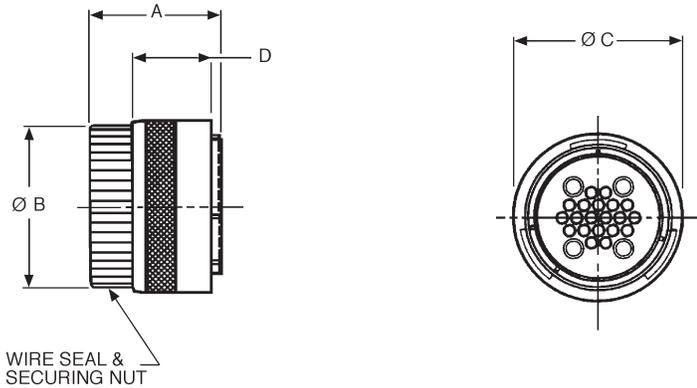
With Wire Seal and Securing Nut
