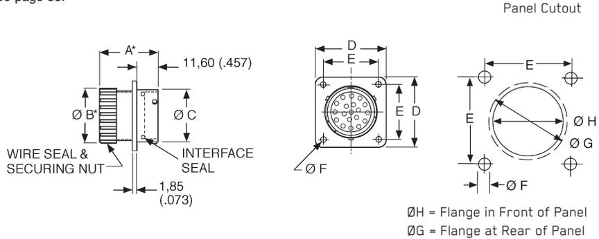
Reversed Receptacles for Pin Contacts Flange Mounting
