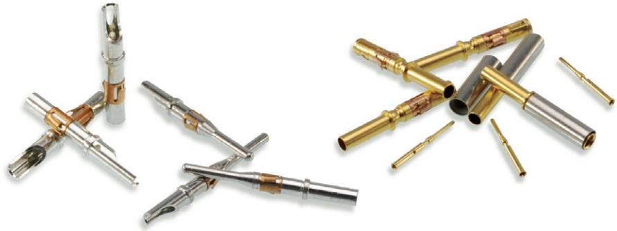
They can be supplied on reels which lowers assembly costs for volume production. Machined contacts offer improved precision and durability. They are recommended for applications with more than 200 mating cycles.
