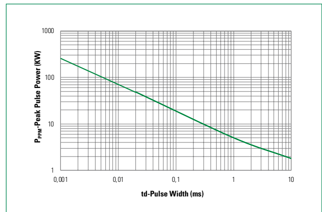
Figure 2: Peak Pulse Power Rating
