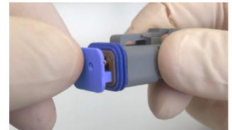
When contacts are in place, insert the appropriate wedgelock until a click is heard. Once male and female housings are prepared the parts can be mated
