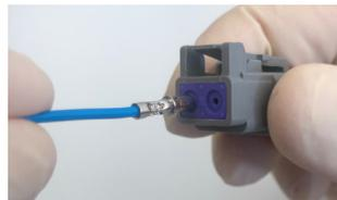
Line the contact up with the grommet.
