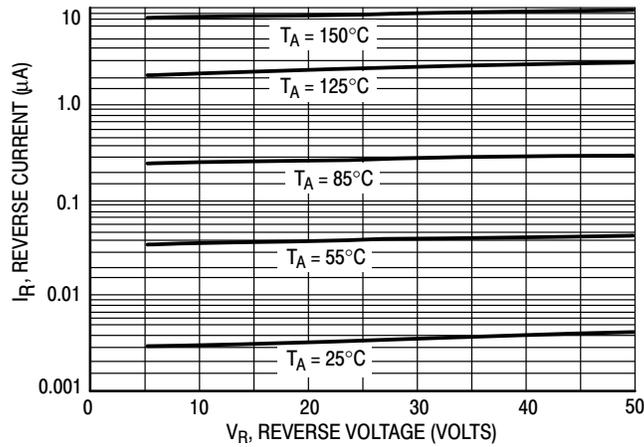
Figure 2. Leakage Current
